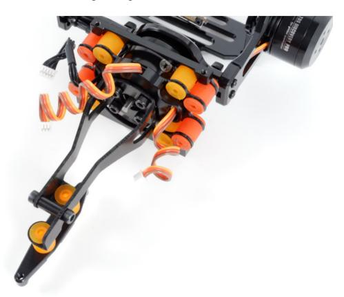
• Mount lever arm with the flat surface with the holes pointing down. The lever plate should have the protruding thread holes also pointing down. This completes the gimbal arm and cage assembly!
