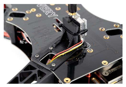
Powerful video transmitters, such as the ImmersionRC 5.8GHz 600mW or more powerful VTx, must be powered directly from the bottom frame (small +/- pads) to avoid overdriving the CORE. Test this a few minutes on the ground and verify that the CORE does not reboot which indicates a thermal protection shutdown/overcurrent.
