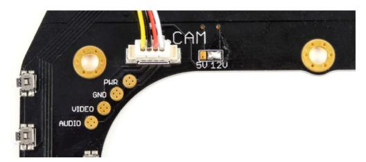
• Plug in the cable connector for the camera and insert the tabs on the top and bottom of the camera frame in the corresponding routed gaps on the frame. For a secure mount, you can add solder to the three exposed solder spots, or leave it for easy hot swapping in the field.
