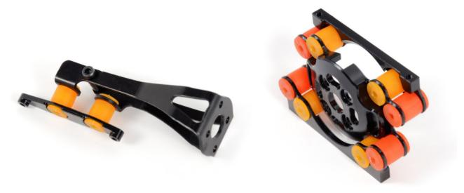
Think of the entire damping layout as accumulating hardness. The green damping balls are the softest, red the medium and orange the hardest. Vary between the colors and layouts, keeping the left and right half of the gimbal symmetrical to find the system that works for you. Top and bottom do not need to remain identical.
